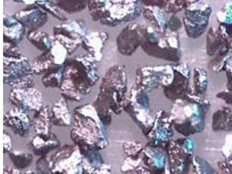
Profilium is a reusable steel abrasive that can be used as a high performance alternative to chilled iron or steel grit. It can also be used as an alternative to expendable abrasives.
