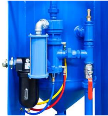
Rear AH-20/24 Pot showing remote control system, and water trap
