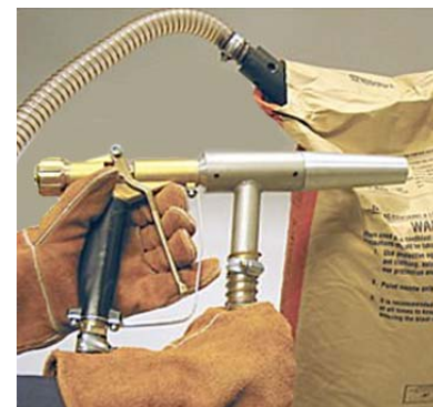
Gun with Suction Tube in bag of abrasive
