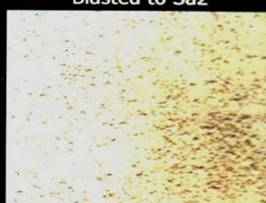
Condition D Blasted to Sa2.5
