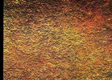
Condition C Unblasted
