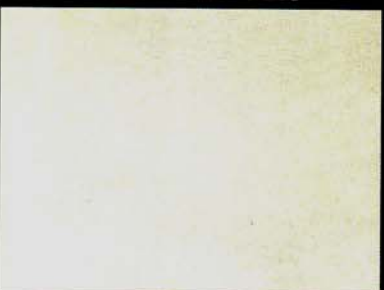
Condition B Blasted to Sa3
