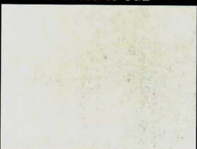
Condition B Blasted to Sa2.5
